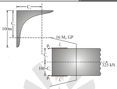
Assuming the thickness of angles as 8 mm, hence minimum size will be 5 cm, because the minimum thickness of thicker part governs the minimum size of weld.
