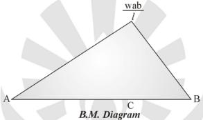
The B.M. diagram for the beam.
